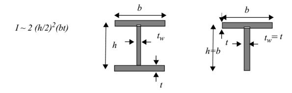
For a beam with a T section as shown above:
